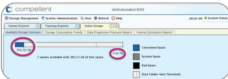
Storage Center advanced virtualization assigns logical disk blocks to logical drives only when data bits are written to the drive. The Dynamic Capacity application builds upon block-level
