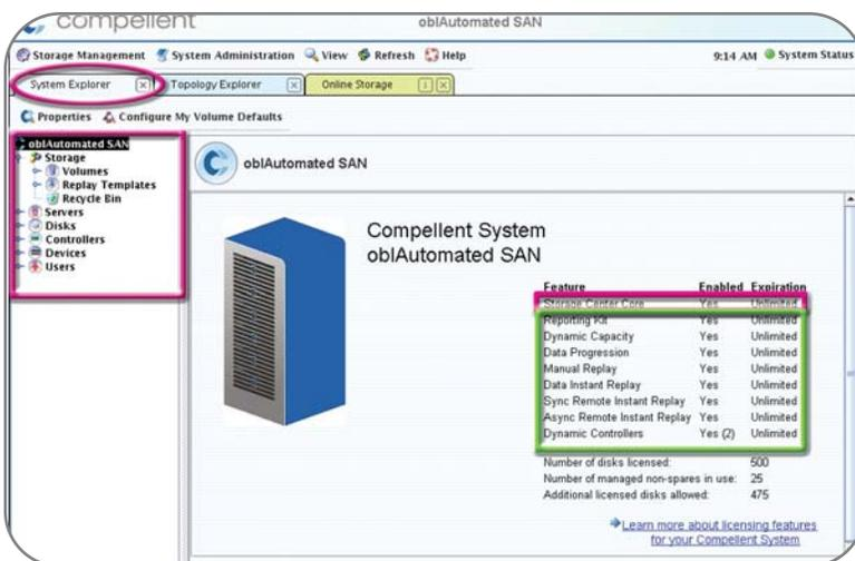
The Compellent Storage Center uses an embedded Web server to provide a single interface that can support all of the SAN’s underlying technology. The classic System Explorer view, uses an expandable tree to present the components that make up the Compellent Storage Center. Also, there is a Topology Explorer view that provides the SAN administrator
