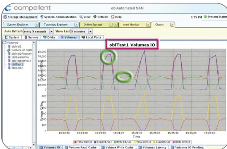
The first logical disk, oblTest1, was created from a pool of Fibre Channel drives spinning at 10,000 rpm. The second logical disk, oblTest2, was created from a pool of SATA drives. Next, we exported both logical drives to an Intel-based server that was running Red Hat Linux.
